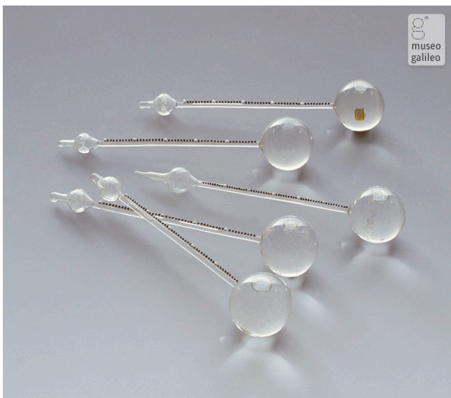
Fig. 1 Thermometers designed by the Grand Duke Ferdinando II de 'Medici, the cinquantigradi thermometers were generally used to learn about the mutations of warm and cold air both outdoors and in closed rooms. The academics made wide use of this type of thermometers, which had the advantage of being comparable between them, especially for systematic meteorological observations.
